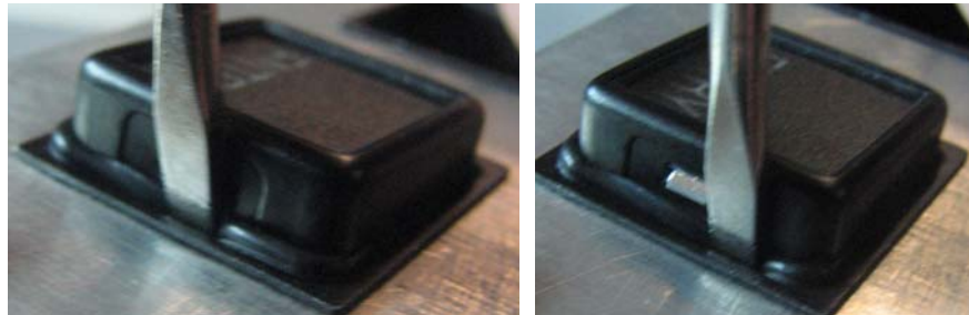
FIGURES 5A & 5B – PUSHING SEAL FROM OUTSIDE TO IN
