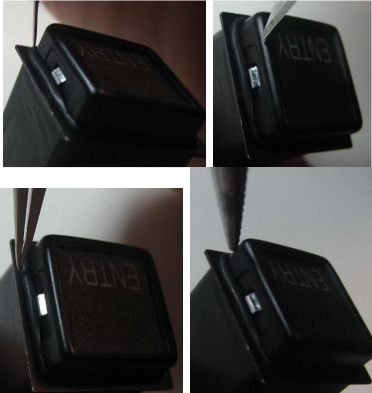
FIGURE 5E – UNACCEPTABLE OBJECTS TO PUSH SEAL WITH
