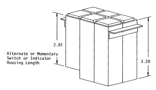
Solenoid Held or Latchdown Switch Housing Length
