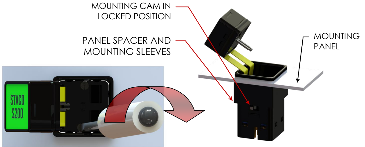
Figure 11: Mounting Cam in Locked Position (flush mount version shown)
