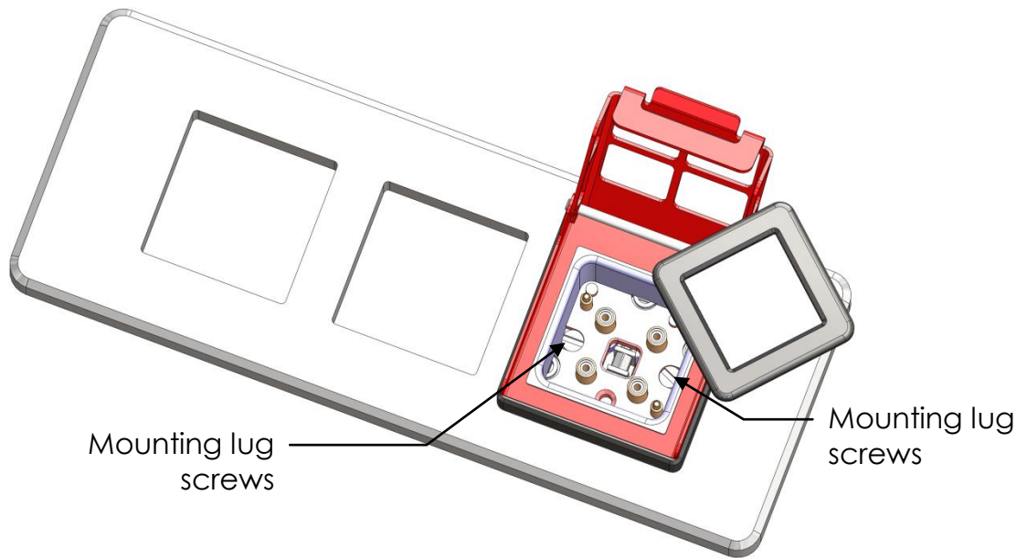
Figure 3: Mounting lug screw details
