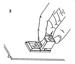
3. Release removal latch and pull pushbutton from matrix housing.
