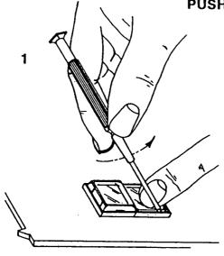
Depress pushbutton until removal latch is free to move. Using small screwdriver or fingernail push removal latch to right and hold.
