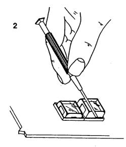
While holding removal latch to right release pushbutton. Spring loaded lamp contacts will push pushbutton to an extended position above matrix and surrounding pushbuttons.
