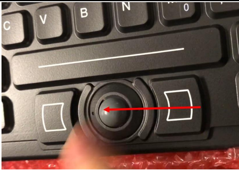
Figure 1 Silicon Rubber Seal Folding as a result of use of short/sharp strikes.
